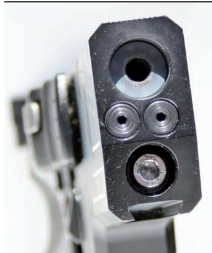
ABOVE: The recoil management system is adjustable via the two hex headed plugs under the muzzle.
