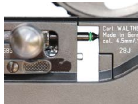
With the bolt action in the 'open' position and the magazine removed, one can clearly see the plunger that pushes a pellet into the barrel.
