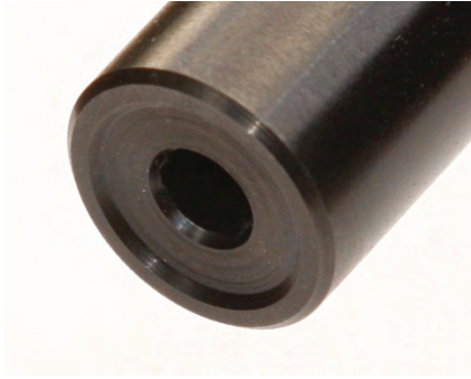
The Venture has a hunting-weight barrel and tapers down to .65" at the muzzle. The target crown is standard.
