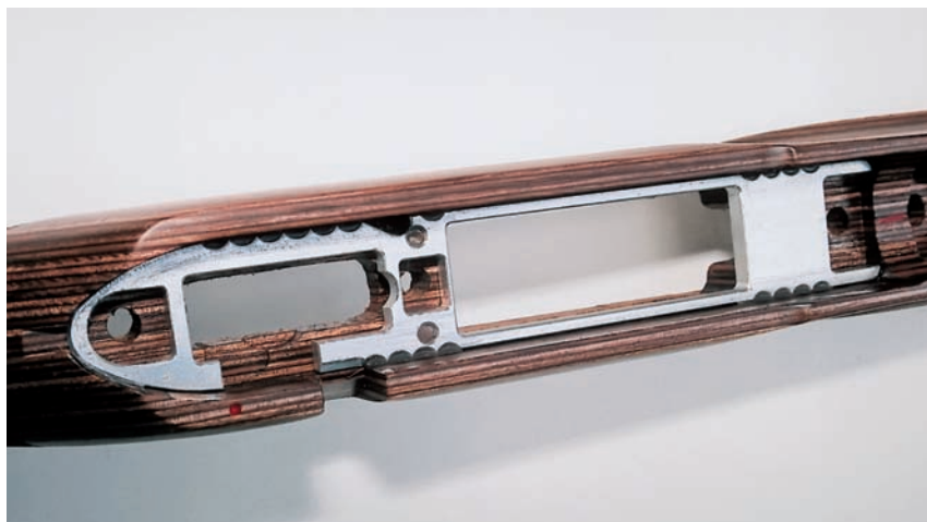
T/C's Interlock bedding system uses a one-piece aluminium block expoxied into the stock on which the receiver sits squarely.
