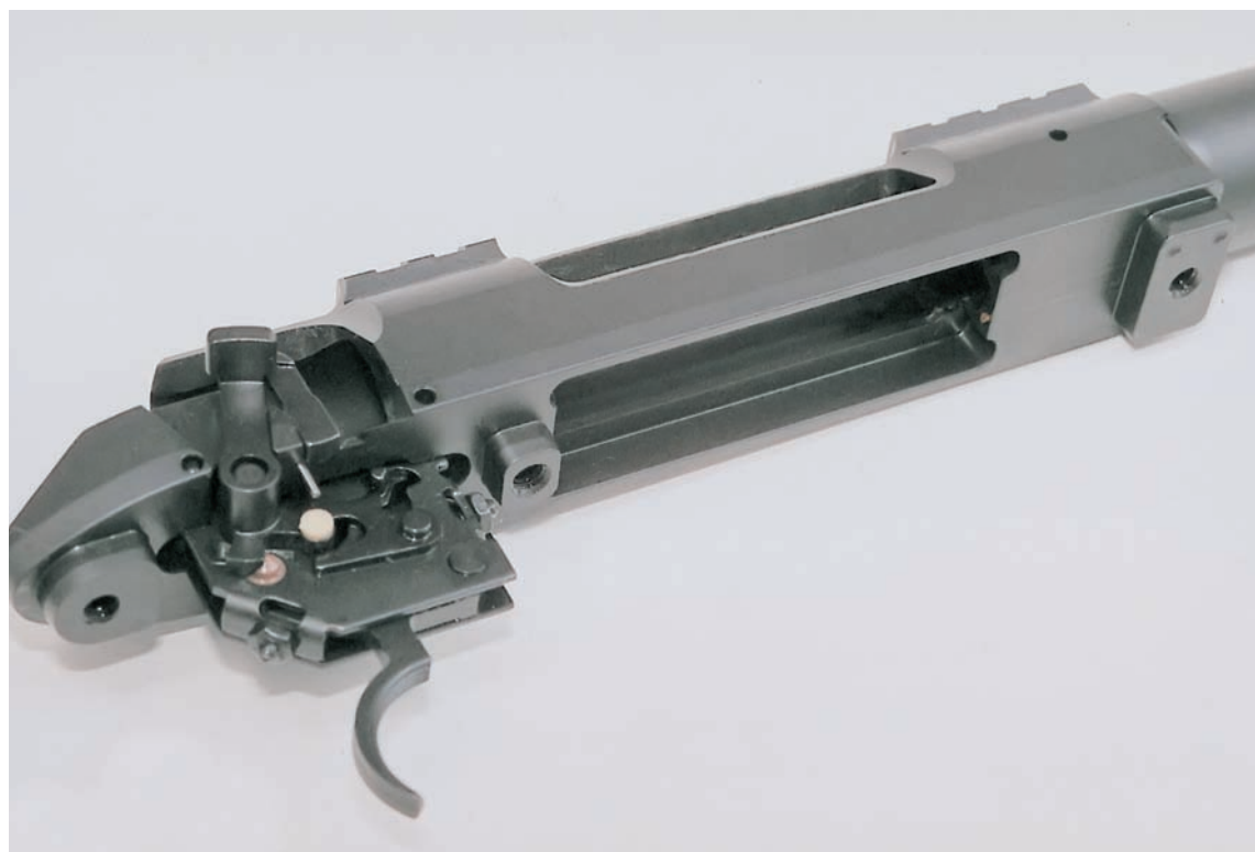
Flat-bottomed receiver has three integral recoil lugs that attach it rigidly to the Interlock bedding block.
